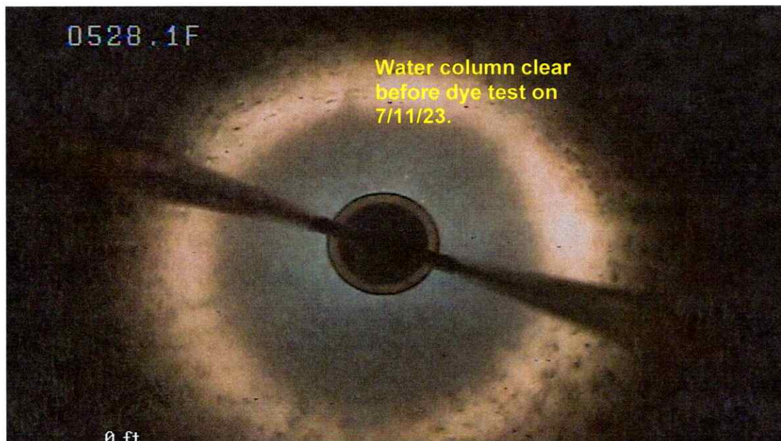
Before Dye Test - 528 feet-bgs
